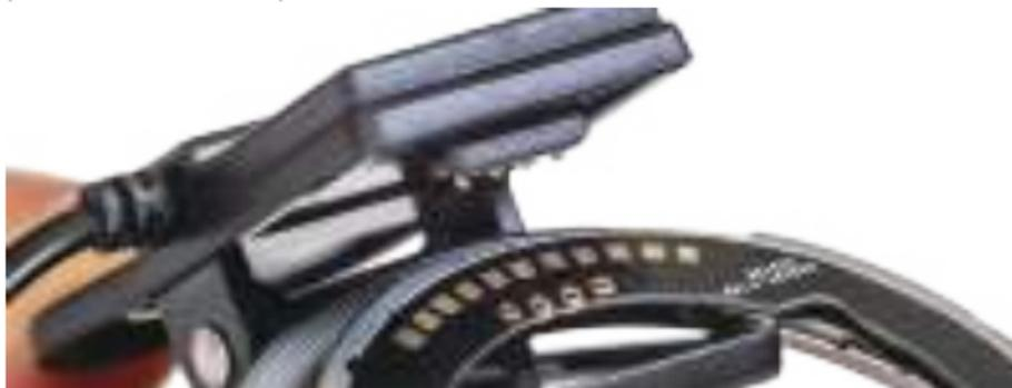
Insert the contact pins while clipping the adapter. Keep a tilted angle to ensure the contact is retained.
